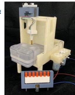
**Luna's FAST platform for rapid electrochemical ELISAs enables IgM and IgG antibody detection, and IgG avidity measurements within an automated microfluidic cartridge and instrument system. Left) ROC curve and distribution plots generated in testing human serum samples of mixed CMV IgG reactivity (N=125, Se. 99%, Sp. 95%). Right) FAST instruments are currently being prototyped with the microfluidic cartridge.**
