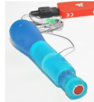
**Luna's prototype handheld device accurately measured stiffness of biological tissue as compared to Instron mechanical tester.**
